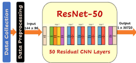
Figure 1 : Pictorial representation of the ResNet 50 Architecture
