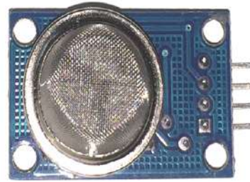
Figure 4: MQ-135 Gas Sensor/Module
