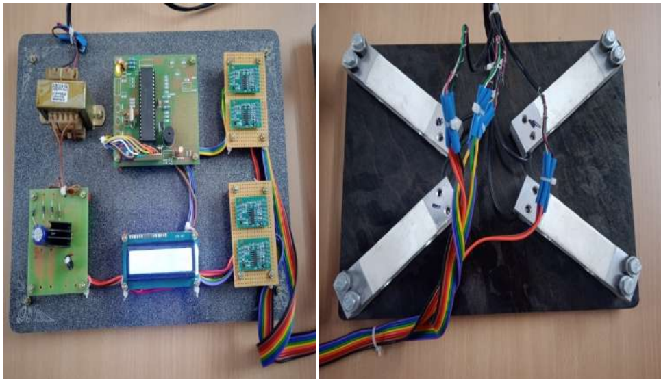
Fig 3: Design Kit - An Analysis and Alert System for Imbalanced Weight Distribution of Sitting Posture
